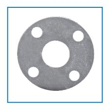
Style 8033 is made of non-asbestos material made by combining aramid and mineral fibers bonded with (SBR) an elastomeric copolymer consisting of styrene and butadiene. It is engineered to have controlled swell properties in oil used in applications throughout the automotive, chemical and industrial processes.
